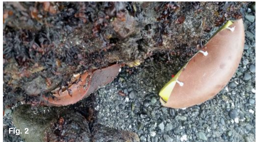
Fig. 2: A live gumboot (left) next to a roboboot (right). Roboboos were an iButton temperature loggers embedded in a carwash sponge and covered by a football skin and attached to the rocks in the intertidal with a vexas mesh and bolts. Roboboos also matched live chitons within 1°C.
