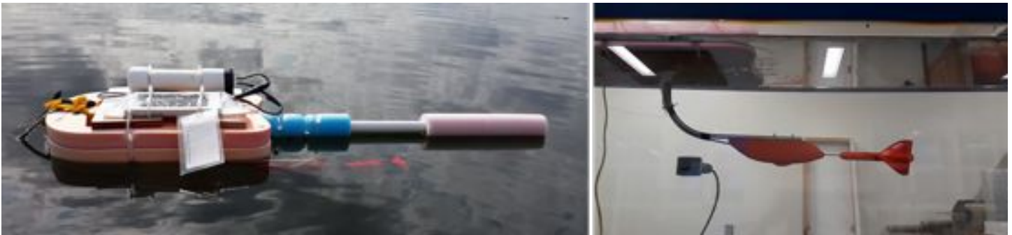
Left - A microcontroller-based current speed sensor deployed in the field. Top view of the sensor. Right - The current sensor suspended in a flow tank at Friday Harbor Labs for calibration. Bottom view of the sensor. Propeller mechanism was constructed from 3D printed components.
